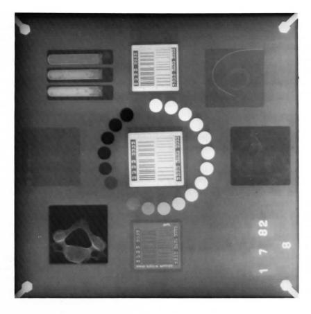
Figure 2.3a. Patient equivalent phantom containing special test objects. A radiograph of the phantom containing test objects shows that both quantitative and qualitative judgments can be made about image quality.
