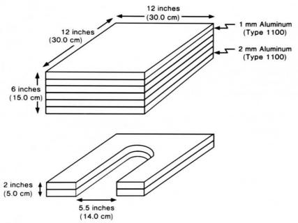
Figure 2.1a. Schematic drawing of the homogeneous patient equivalent phantom (PEP). The phantom and base, made of acrylic and aluminum, are used extensively in a quality control program.
