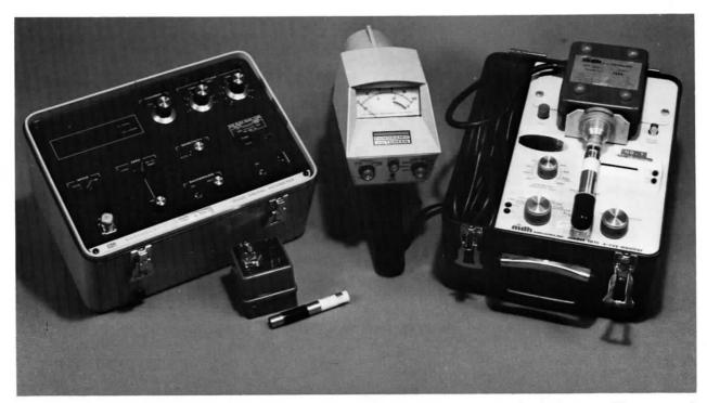
Figure 2.4. Radiation measurement equipment. The survey meter (center) is not suitable for dosimetry or QC purposes. A pen dosimeter, shown in the lower left with its charger-reader, can be used for limited purposes, but because of its inherent limitations we do not feel it is accurate enough for QC purposes. Direct readout dosimeters (on the left and right), although somewhat costly, are essential for reliable and accurate dosimetry and for a good QC program.
