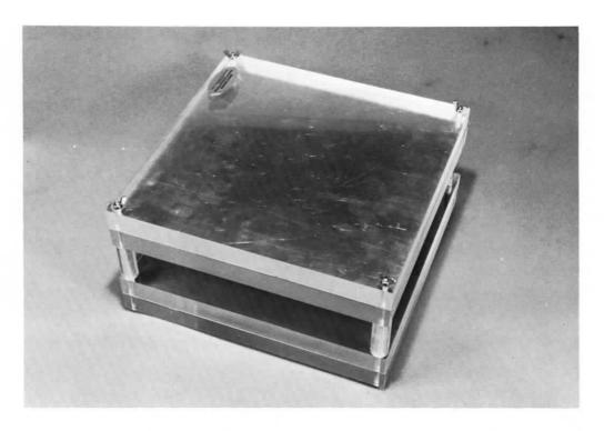
Figure 2.2a. PEP for chests and extremities. The basic PEP can be modified to provide a phantom that simulates the chest and extremities. The chest phantom is similar to the basic phantom, but two slabs of acrylic [2 inches (5 cm)] are removed from the center. A 2-inch (5-cm) air gap is left between the remaining layers.
