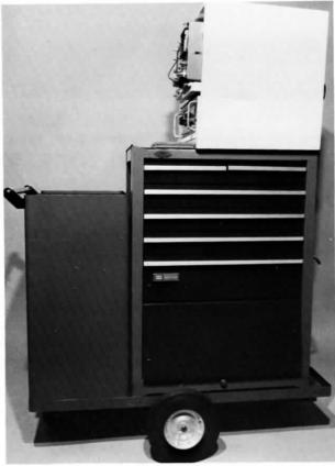
Figure 2.6b. All QC test tools are contained in the locked drawers and lower storage area (including the PEP). One small drawer is lead-lined so that film can be stored in the cart without risking film fog. The flat area to the left provides a writing area. Various ionization chambers are stored in one drawer, which has been lined with foam containing cutouts to fit each chamber.
