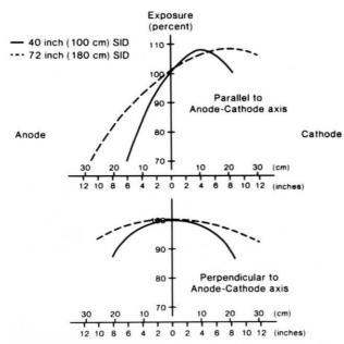
Figure 2.8. The heel effect can cause difficulty in making radiation measurements. Considerable variability will be noted as the ionization chamber is moved parallel to the anode-cathode axis, expecially with a 40-inch (100-cm) SID. Variation is not nearly as significant perpendicular to the anode-cathode axis, but it is still present.
