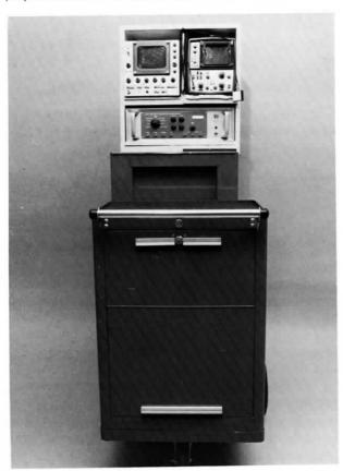
Figure 2.6a. Quality control equipment cart. It is convenient to have all of your equipment on one cart so that it is available when you are working in a room. The locked section contains tools (screwdrivers, pliers, etc.) and the readout section of the dosimeter. The rack on top was added to the cart to hold electronic test gear.
