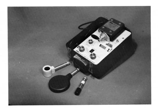
Figure 2.5a. For QC purposes we recommend a direct readout digital dosimeter that digitizes the signal at the ionization chamber. Three chambers are necessary for specific purposes: a thin-windowed chamber for mammography (left); a large volume chamber for use under phantoms and in making measurements at low radiation levels (center); and a small volume chamber for making measurements at high radiation flux levels as well as monitoring the x-ray waveform (right).
