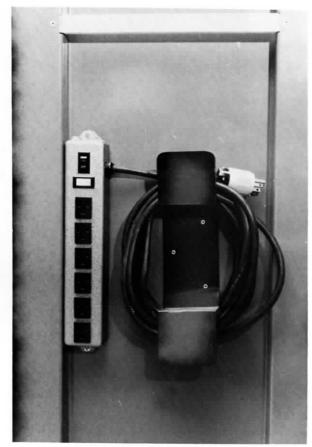
Figure 2.7. Multiple outlet box. Since most radiographic rooms do not have sufficient outlets to support all of the test gear, and to make set-up easier and quicker, a multiple outlet box with a switch and circuit breaker is mounted on the right side of the cart (relative to Figure 2.6b). In addition, an extra-long electrical cord is provided so that the cart can be positioned anywhere in the x-ray room.
