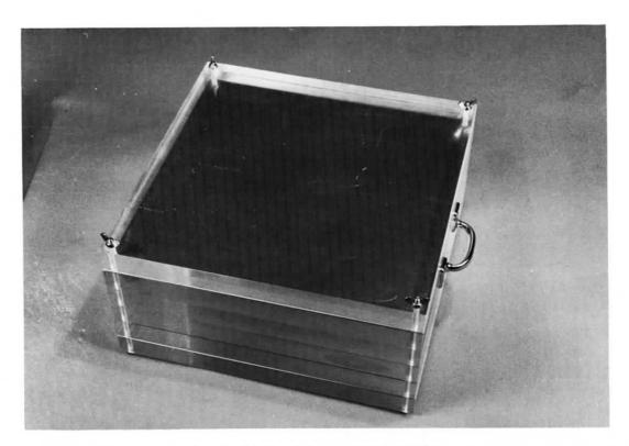
Figure 2.1b. Basic PEP, which is used to simulate the abdomen, skull, and pelvis.
